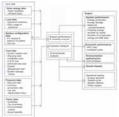
Figure 7 : Flow chart of model used to make economic, environmental and social assessments of three types of electricity sources.
